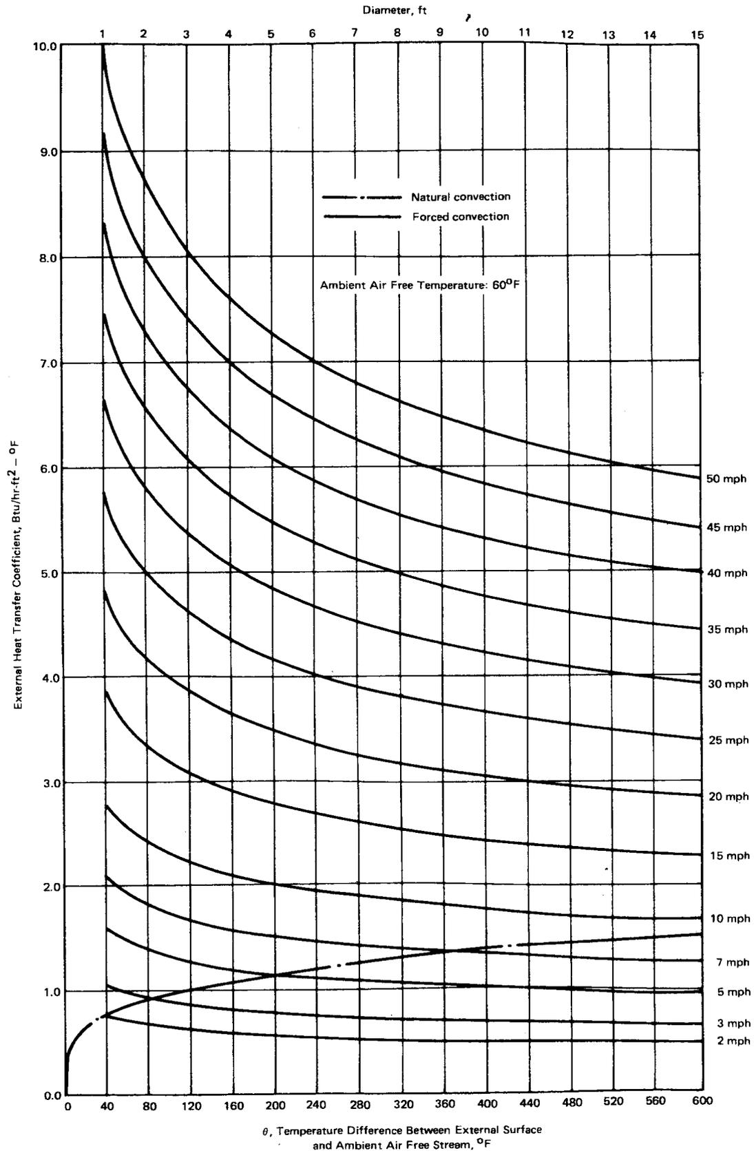
Figure B2-1 - External heat transfer coefficient for forced and natural convection
