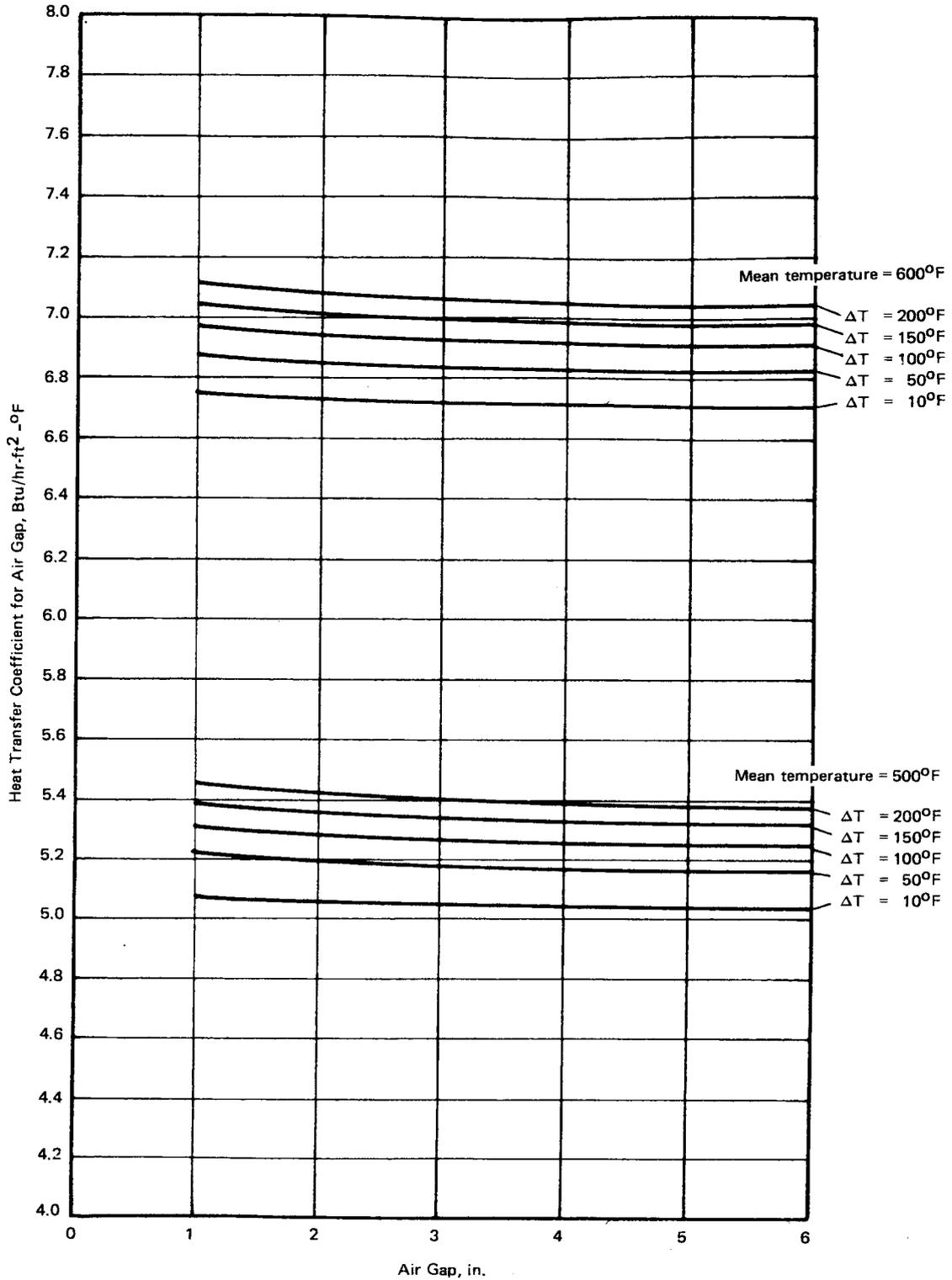
Figure B2-4 – Heat transfer coefficient for the air gap between two walls of a double-walled metal chimney
