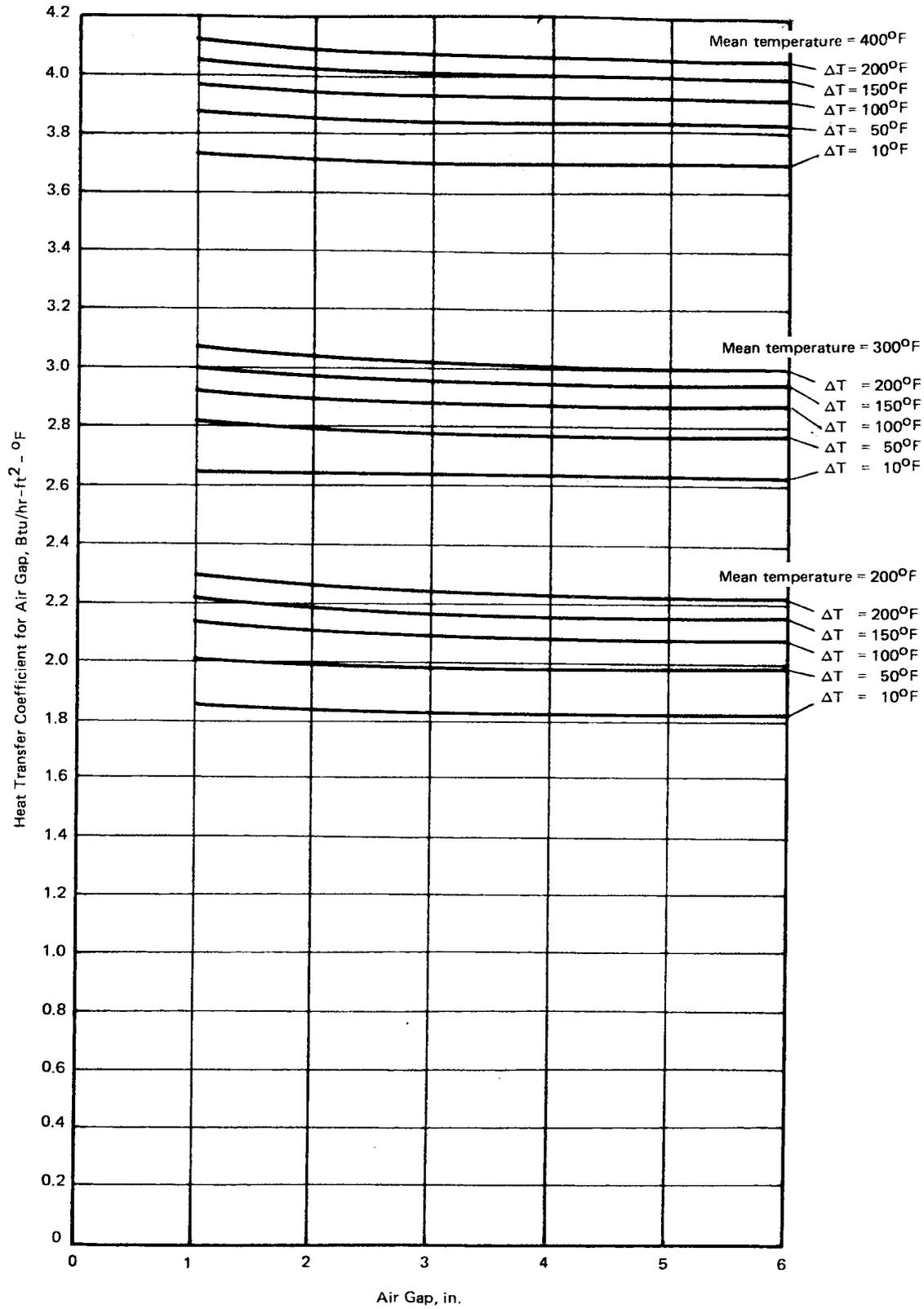
Figure B2-3 - Heat transfer coefficient for the air gap between two walls of a double-walled metal chimney (courtesy of Warren Engineering, Inc.)
