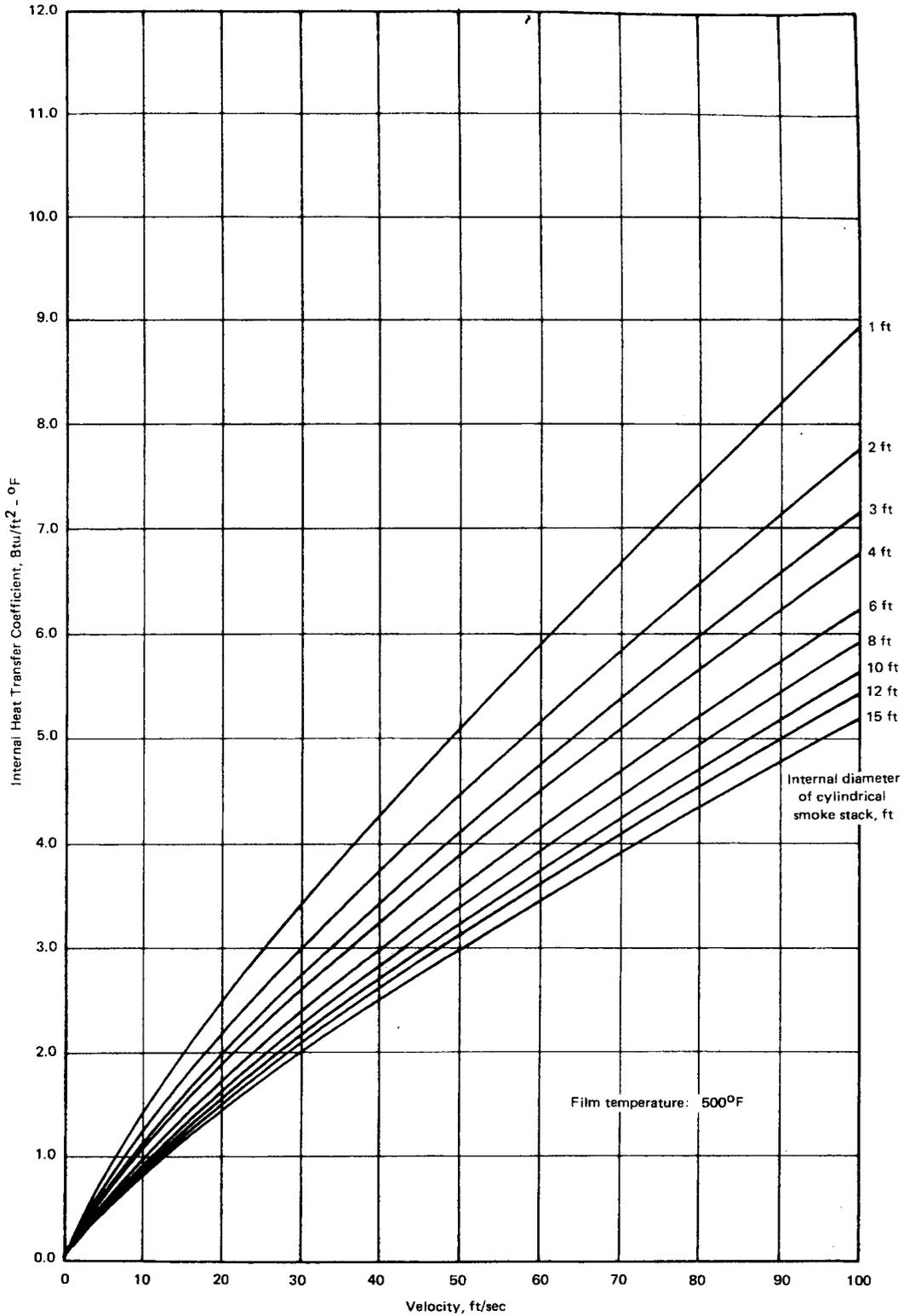
Figure B2-7 - Internal heat transfer coefficient (Btu/hr-ft<sup>2</sup>-°F) vs. velocity (ft/sec)
