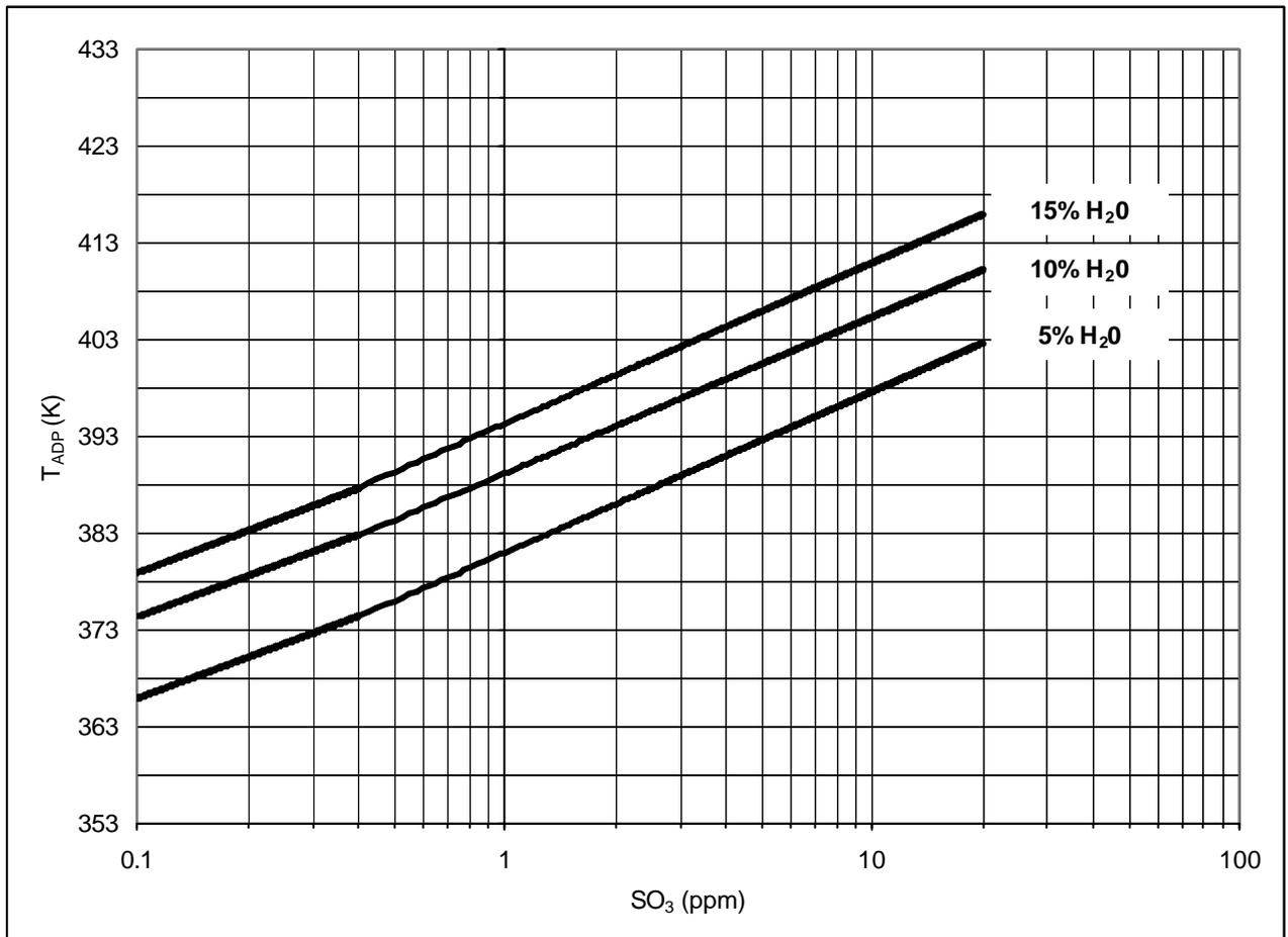
**Figure C1 - Temperature of the acid dew point, T<sub>DP</sub>, of gases containing water vapour (H<sub>2</sub>O) and sulphur trioxide (SO<sub>3</sub>)**
