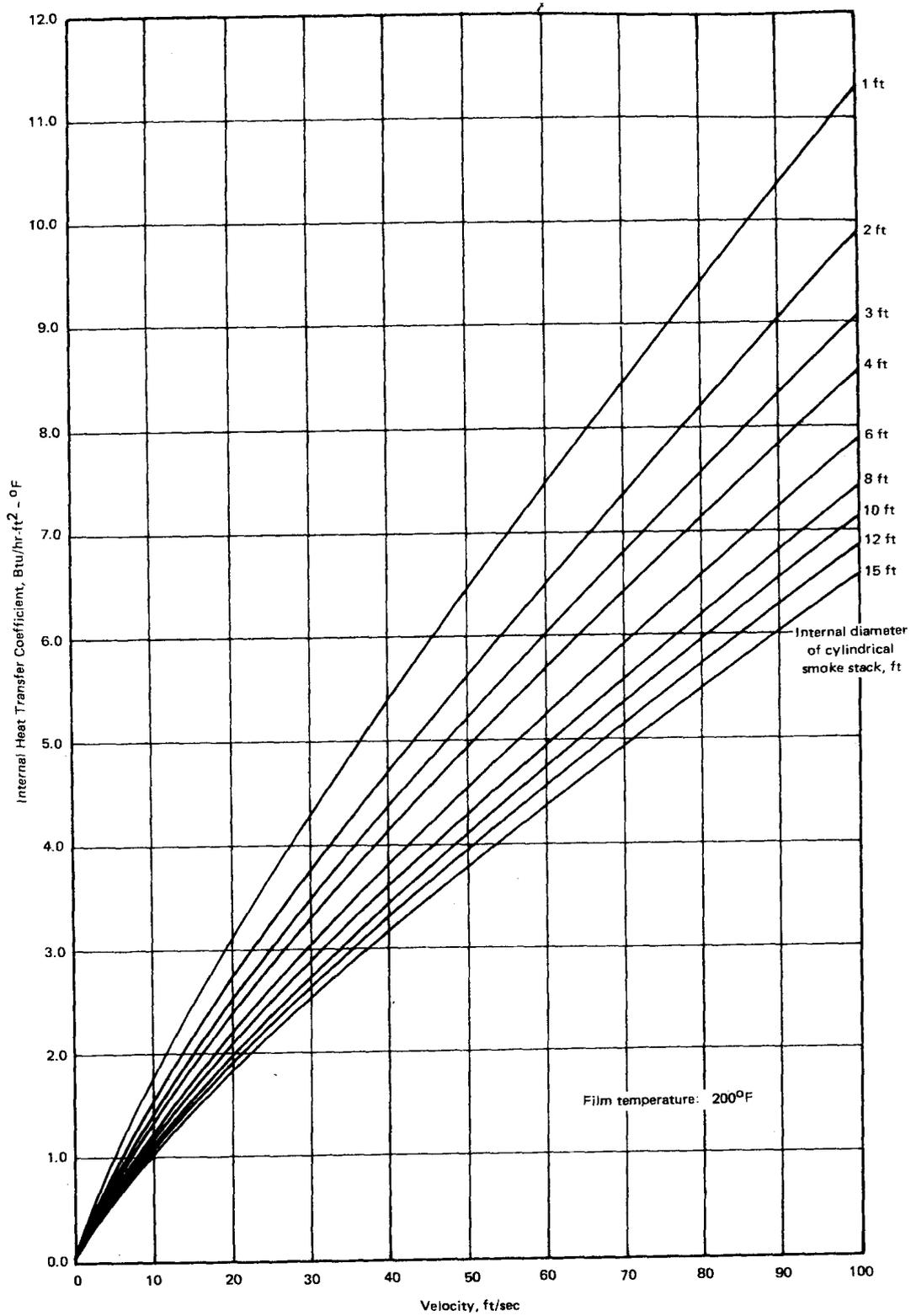
**Figure B2-5 - Internal heat transfer coefficient (Btu/hr-ft<sup>2</sup>-°F) vs. velocity (ft/sec)**
