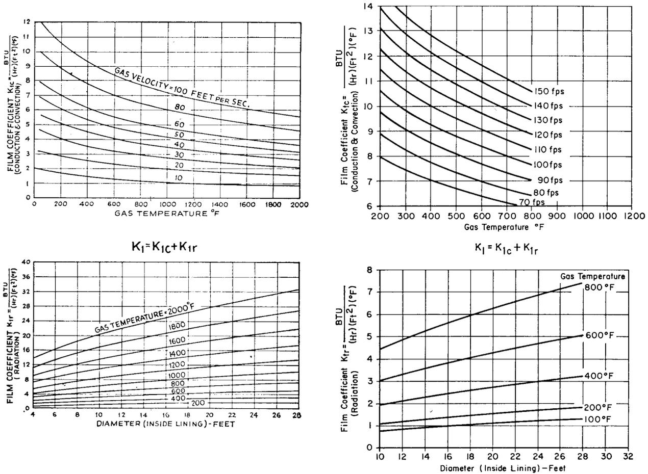
Figure B1—Flue gas film coefficients (from ACI 307)
