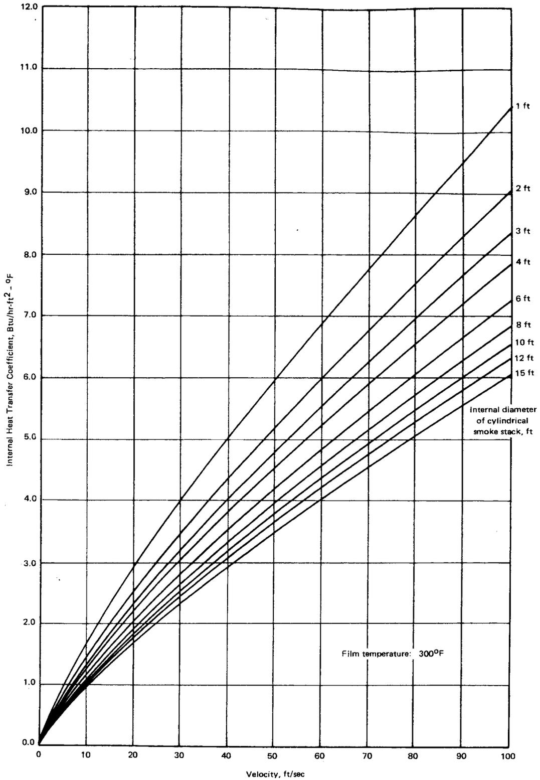
Figure B2-6 - Internal heat transfer coefficient (Btu/hr-ft<sup>2</sup>-°F) vs. velocity (ft/sec)
