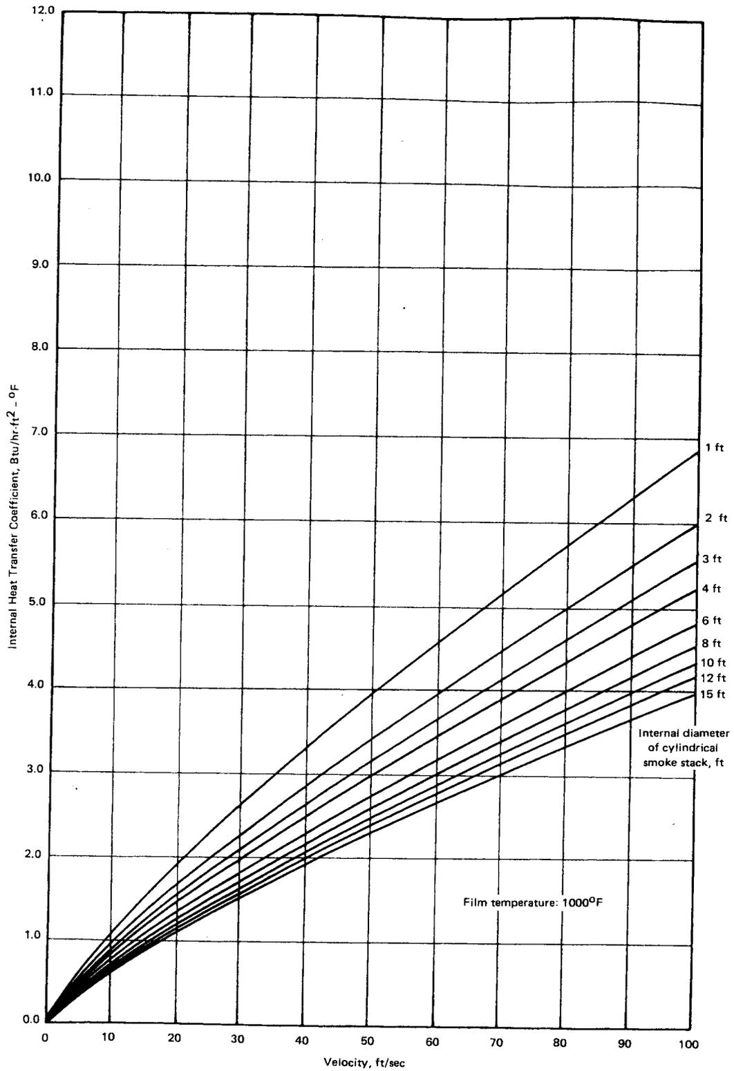
Figure B2-8 - Internal heat transfer coefficient (Btu/hr-ft<sup>2</sup>-°F) vs. velocity (ft/sec) - film temperature of 1000°F (courtesy of Warren Engineering, Inc.)
