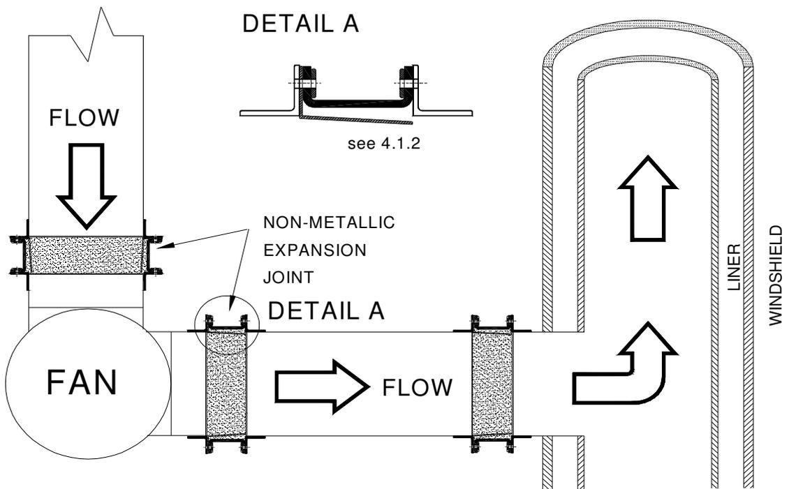
Figure 2 - Non-metallic expansion joint
