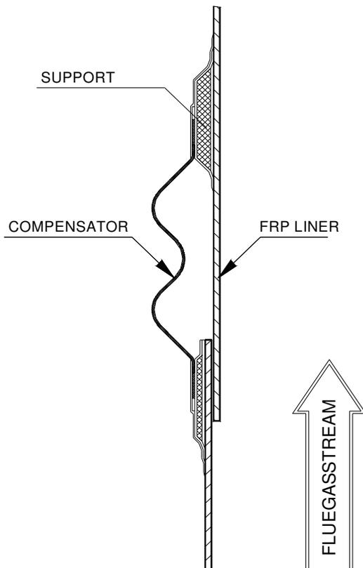
Figure 16 FRP liner seal
