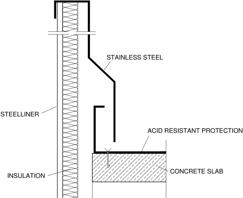
Figure 14 Weather Hood Seal
